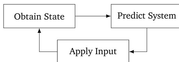
Figure 1.1: Illustration of the model predictive control cycle.
